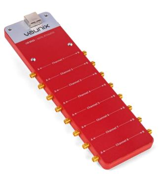
The Lab Brick LDA series of Digital Attenuators bring affordability, functionality, reliability, and simplicity to the microwave test bench. The LDA products range from 6 MHz to 40 GHz with input level tolerance to 2 Watts and step size as small as 0.1 dB.
