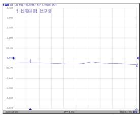
In IL test setup, two Waveguide to Coax Adapters are connected together
